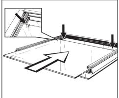
Slide the middle pane in slightly and then refit the seal. Then push the pane right in.
